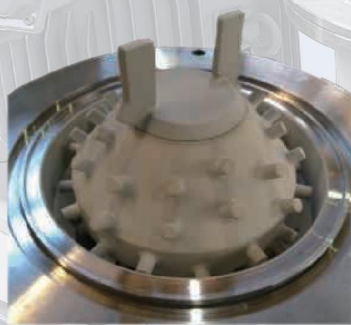
Alumina thermal spray coating on rotor and casing inner wall
